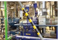
VKO 725S for the compression of lime kiln gas with turbine drive - year of construction 1976.
